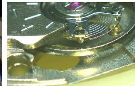
4. Using sturdy tweezers, set the stud to the stud support and press it down.
