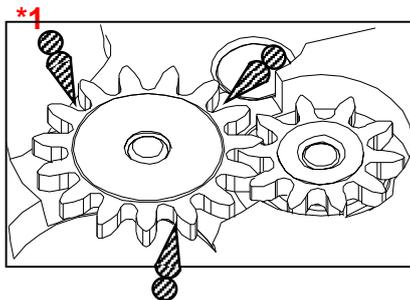
Barrel and train wheel bridge (back side)
