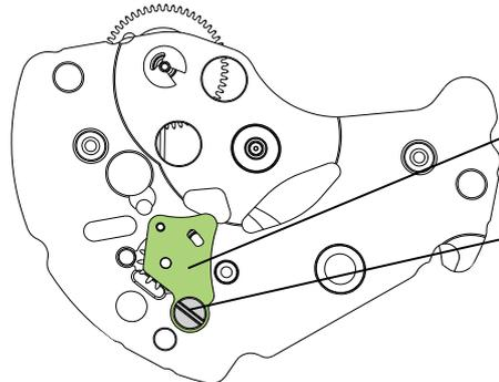
③5 Lower plate for barrel and train wheel bridge
