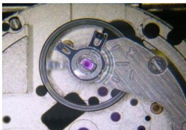
3. Using sturdy tweezers, push the stud outward from the direction of the arrow shown in the illustration until it is removed from the stud support.
