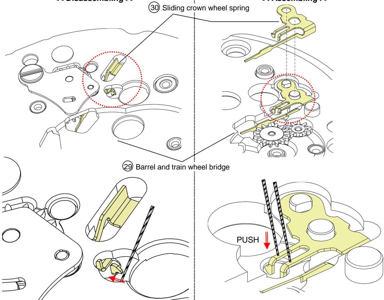
Remove the hook of the Sliding crown wheel spring from Barrel and train wheel bridge.
