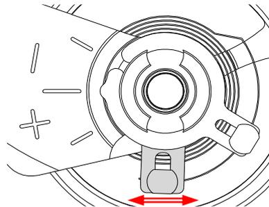
•Regulator pin ... Gap adjustment of balance spring and regulator pin
