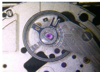
3. Temporarily set the stud to the stud support. Make sure that the balance spring passes outside the regulator pin.
