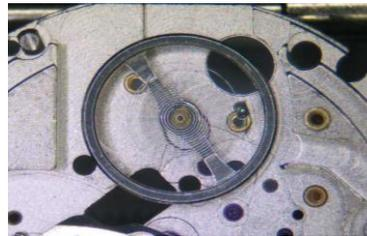
2. Set the Balance cock and tighten the balance cock screw.
