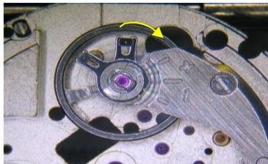
2. Make sure that the outer coil is not removed from the regulator arm.
