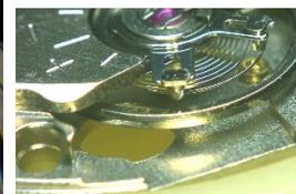
4. Using sturdy tweezers, set the stud to the stud support and press it down.
