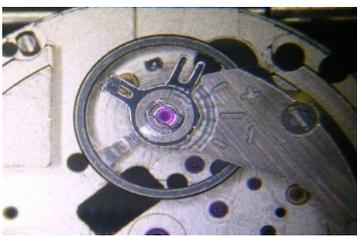
4. Unscrew the Balance cock screw and remove the Balance cock.
