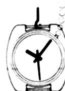
If there is a defect in water resistance somewhere, air inside the watch case bubbles out there.
