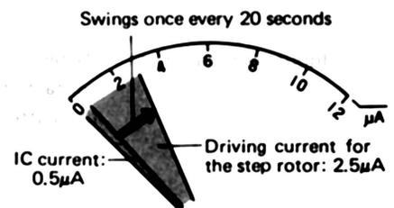
**Note:** In the case of those watches with the minute hand moving at 5-, 10-, or 30-second intervals, calculate their current consumption accordingly on the basis of the above example.
